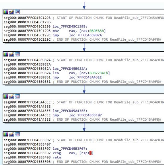
Figure 44: Process that bfcsvc.dll uses to call DLL function.
